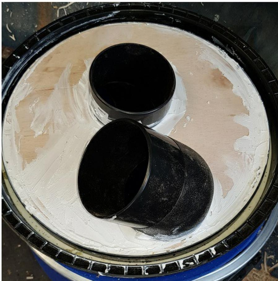
“Slavered the whole plywood edge, and around the 100mm pipes with sealant”.
