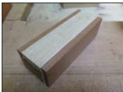
*The sides glued on, (using a different but still dark material to show up the 'wings'), ready for another 24 hours resting in the vice*
