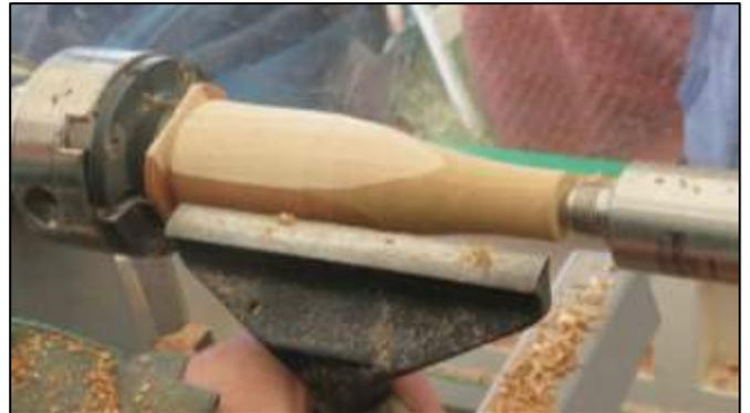
2 turning the basic shape shows the difference in height of the wings (darker) and the breast (lighter)
