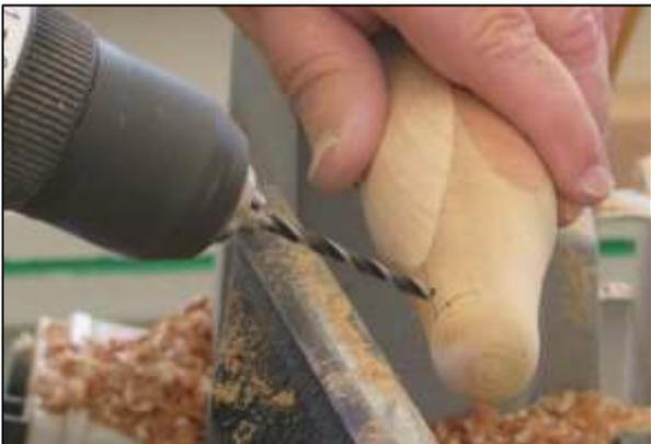
5 A spur point drill (4mm) is used for the beak, while a 3mm drill is used for the eyes. (if you use a 4mm for the eyes, they fall in!) Great care and accuracy needs to be achieved at this point, or the penguin will acquire the unfortunate name of Isaiah.
