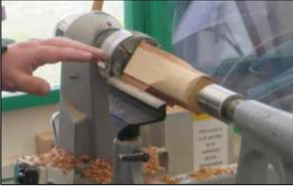
1 Roughing out the shape clearly shows the reduction in the width of the wings.
