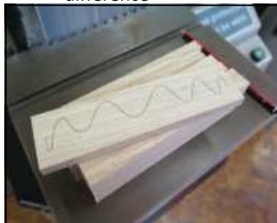
*The pencil squiggle enables you to see if the whole surface is correctly flattened ready for gluing*
