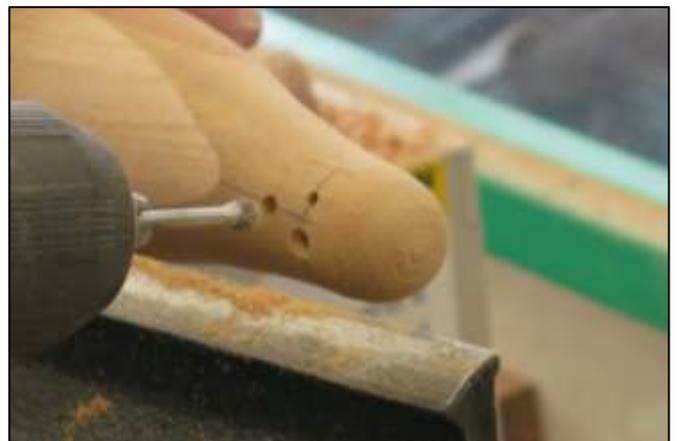
6 The eye sockets are shaped using a 6mm burr, to about a third of the depth of the burr. Both eyes must be equal in depth
